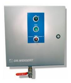
Dosing equipment for cleaners and disinfectants, wall units. Two cleaning respectively disinfecting concentrates can be connected to one unit. Dosage via integrated metering pumps. Solutions can be taken directly from the outlet tap or sprayed with a spray lance. Mount in a central position on the wall. 10-metre long pressure hose makes it possible to carry out cleaning even in distant locations.
