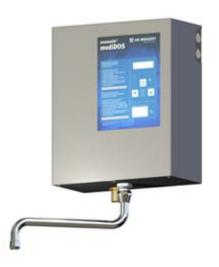
The microprocessor-controlled dosing device serves to produce ready-to-use detergent and disinfectant solutions from liquid concentrates for manual application. The mixing device with a robust stainless steel casing for wall mounting can be easily operated and features an automatic switch-off in the case of product depletion as well as fill level monitoring.
