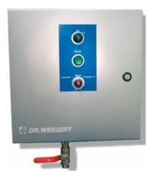
Dosing equipment for cleaners and disinfectants, wall units. Two cleaning respectively disinfecting concentrates can be connected to one unit. Dosage via integrated metering pumps. Solutions can be taken directly from the outlet tap or sprayed with a spray lance. Mount in a central position on the wall. 10-metre long pressure hose makes it possible to carry out cleaning even in distant locations. neomatik® SGW 1 (for one product) neomatik® SGW 2 (for two products)
