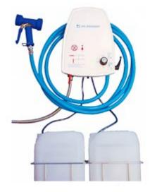
Stationary wall spray unit for the manufacturing and spraying of ready-for-use cleaner and disinfectant solutions. Two cleaning respectively disinfecting concentrates can be connected to one unit. Dosing via an injector, with spray gun, canister holder and 20 m pressure hose. Mount in a central position on the wall.
